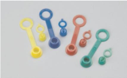
Grease fitting caps snap securely over grease fittings to seal out dirt and moisture. Integral retaining ring keeps cap in place during servicing. Choose from red, orange, yellow, green, blue, and purple to indicate grease type or relubrication frequency. Available in two sizes to fit 1/8 NPT or 1/4-28 zerk fittings. Sold in bags of 10 caps, all one color.
