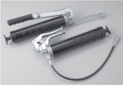
Trico's grease guns are built using aluminum die cast heads and are available in rugged lever or pistol grip versions. The pistol grip version comes with a flex hose and is capable of developing 5,000 psi grease pressure. The lever version comes with a rigid nozzle and is capable of developing 10,000 psi grease pressure. Trico's grease guns are to be used with 14 ounce grease cartridges.
