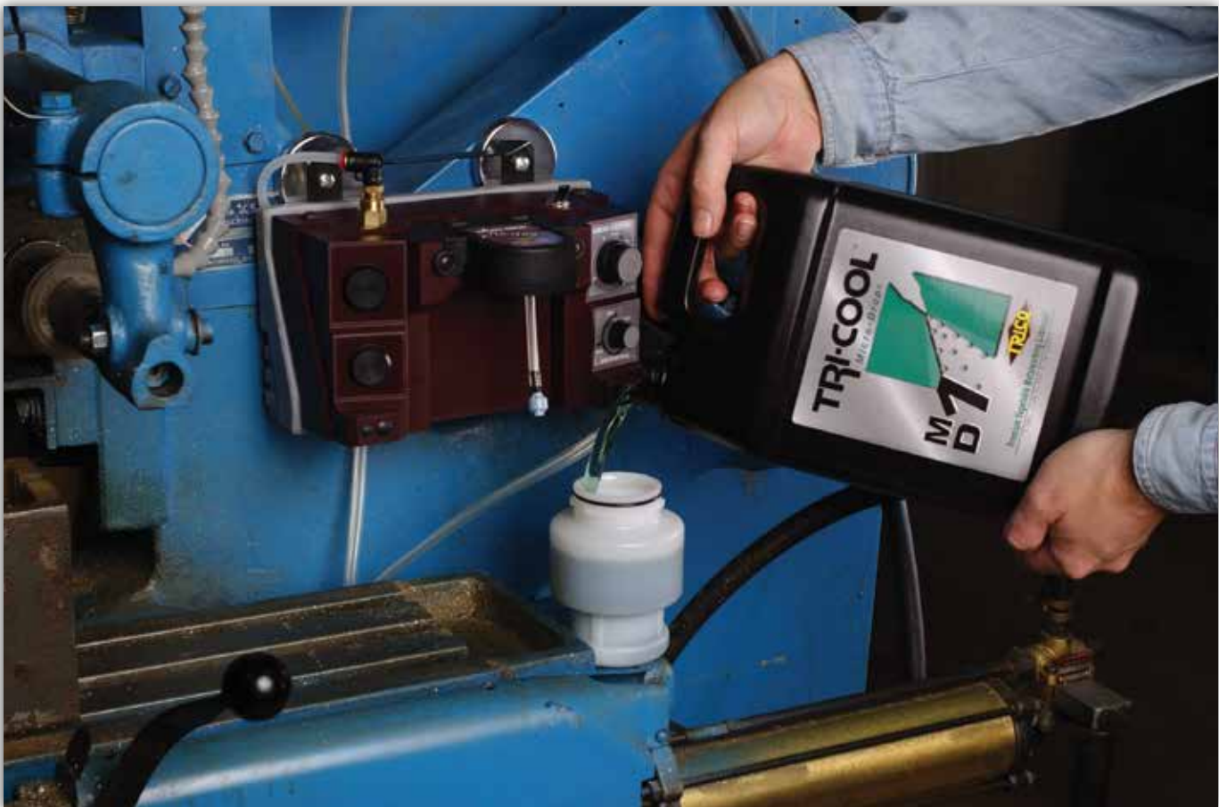
Micro-dispenser being filled with Tri-Cool MD-1 lubricant
