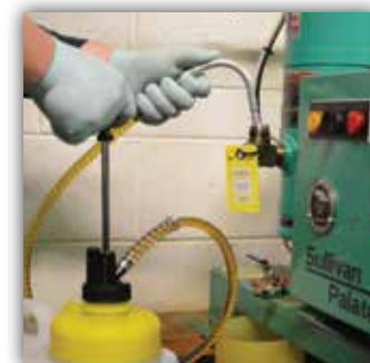
Compressor being filled with a Spectrum Container using the hand pump
