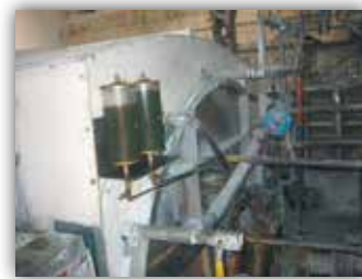
Gravity feed oilers on a mud washing drum
