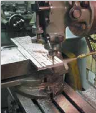
Spray cooling during milling operation
