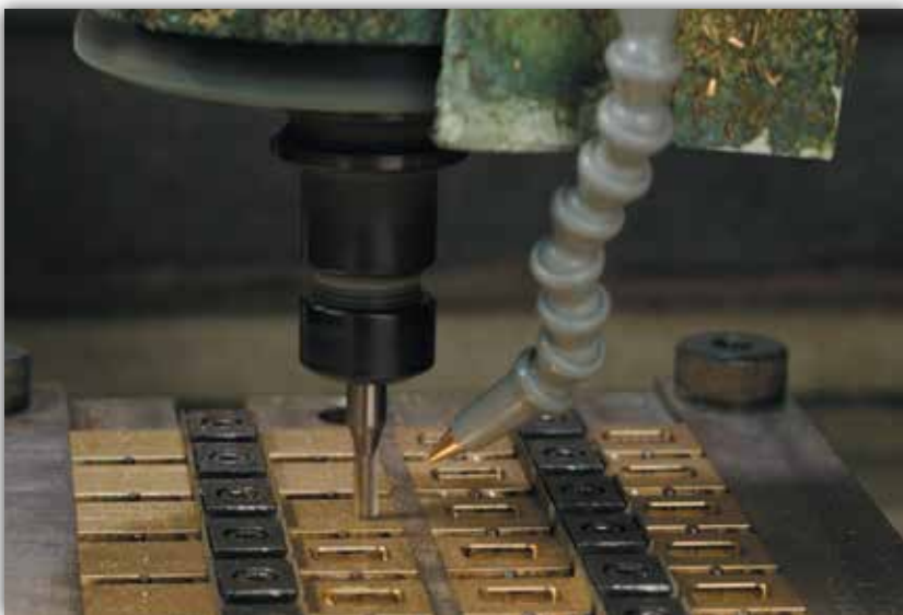
Minimum quantity lubrication used during a milling operation
