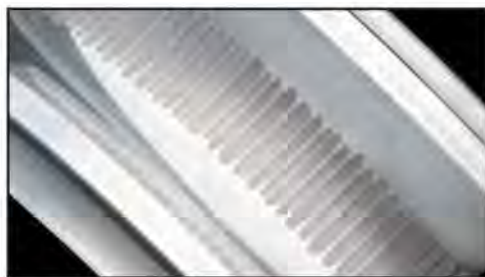
Stray shaft currents can cause fluting on the bearing race, resulting in premature bearing failure.
