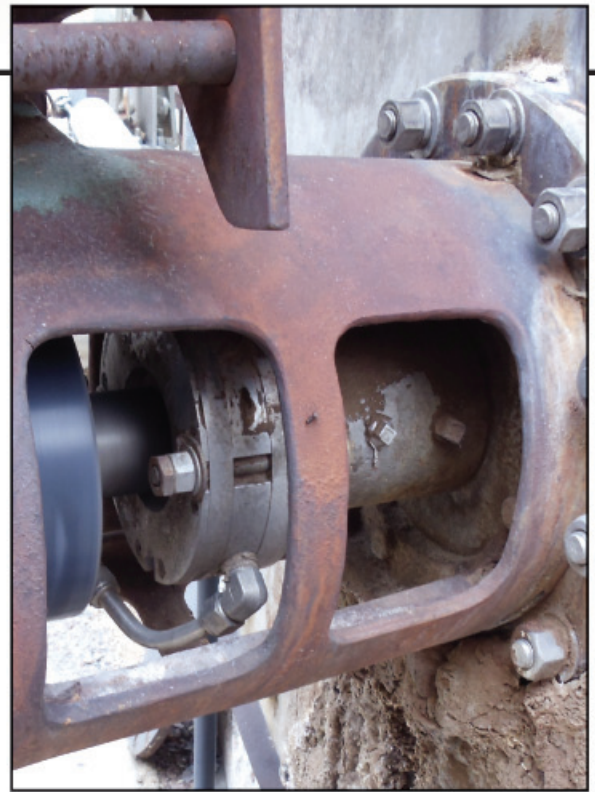
A stainless steel Air Mizer seal installed on a side entry agitator eliminates product waste and contamination.
