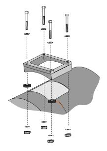
Secure window frame to guard body with provided fasteners. Two neoprene washers are provided to be used as spacers should position of window frame straddle adjustment seam on barrel of guard. Once Frame has been secured to guard slide window into place and secure with supplied fastener.
