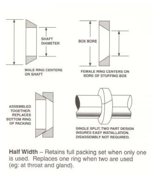
To Order: Supply inside diameter (i.d.) x outside diameter (o.d.) x cross section of packing box and state full or half width.
