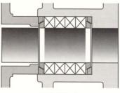
TWO SELF-ADJUSTING THROAT BUSHINGS ONE INSTALLED AT EACH END OF STUFFING BOX
