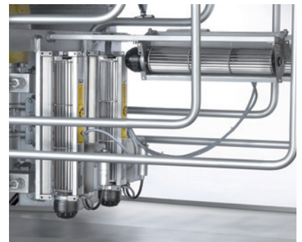
Tangential blowers to cool valve cylinders
