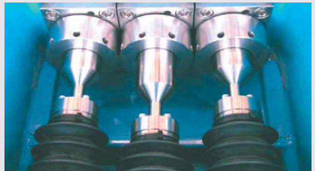
The bellow-type seal of the ABEL HPT pump reliably protects the gear against contamination by dirt and fluids
