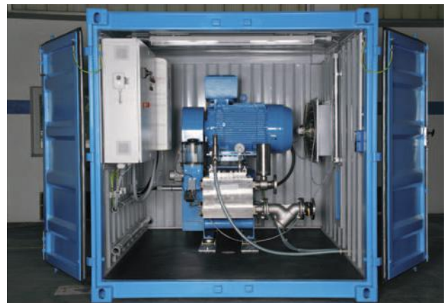
ABEL HPT as ready-to-use, mobile container pump
