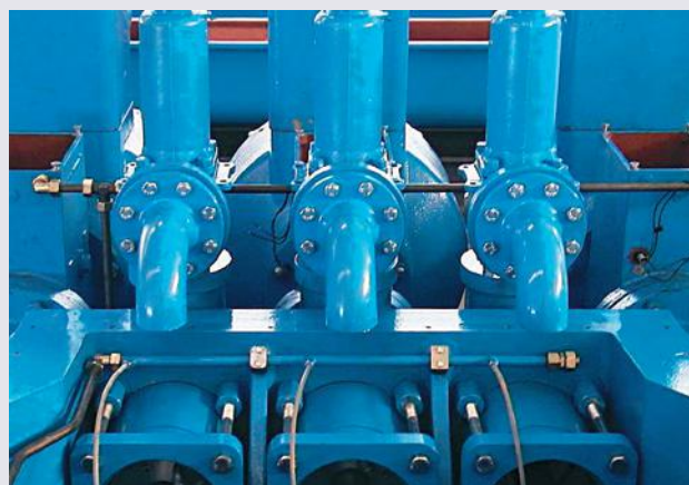
Full-stroke pressure relief valves on the hydraulic side
