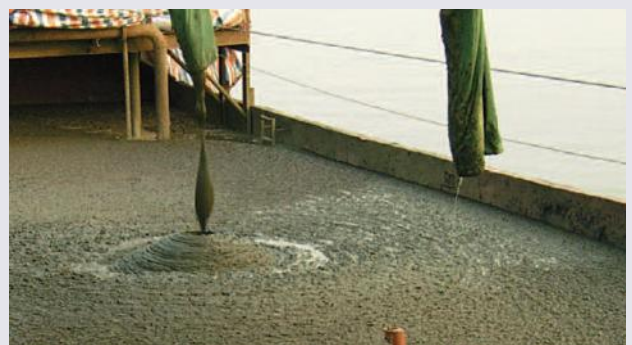
Thickened, digested sewage sludge, 7 % solids concentration
