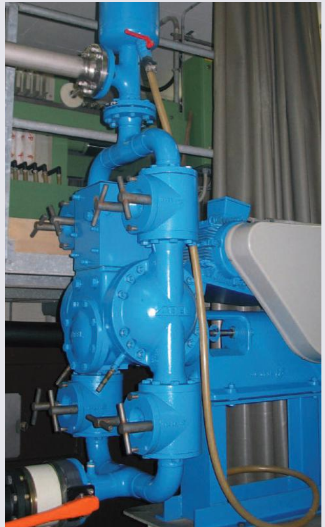
Ball valves with inspection opening and diaphragm leakage detection device
